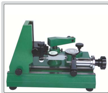
Inspect accuracy of test indicators
